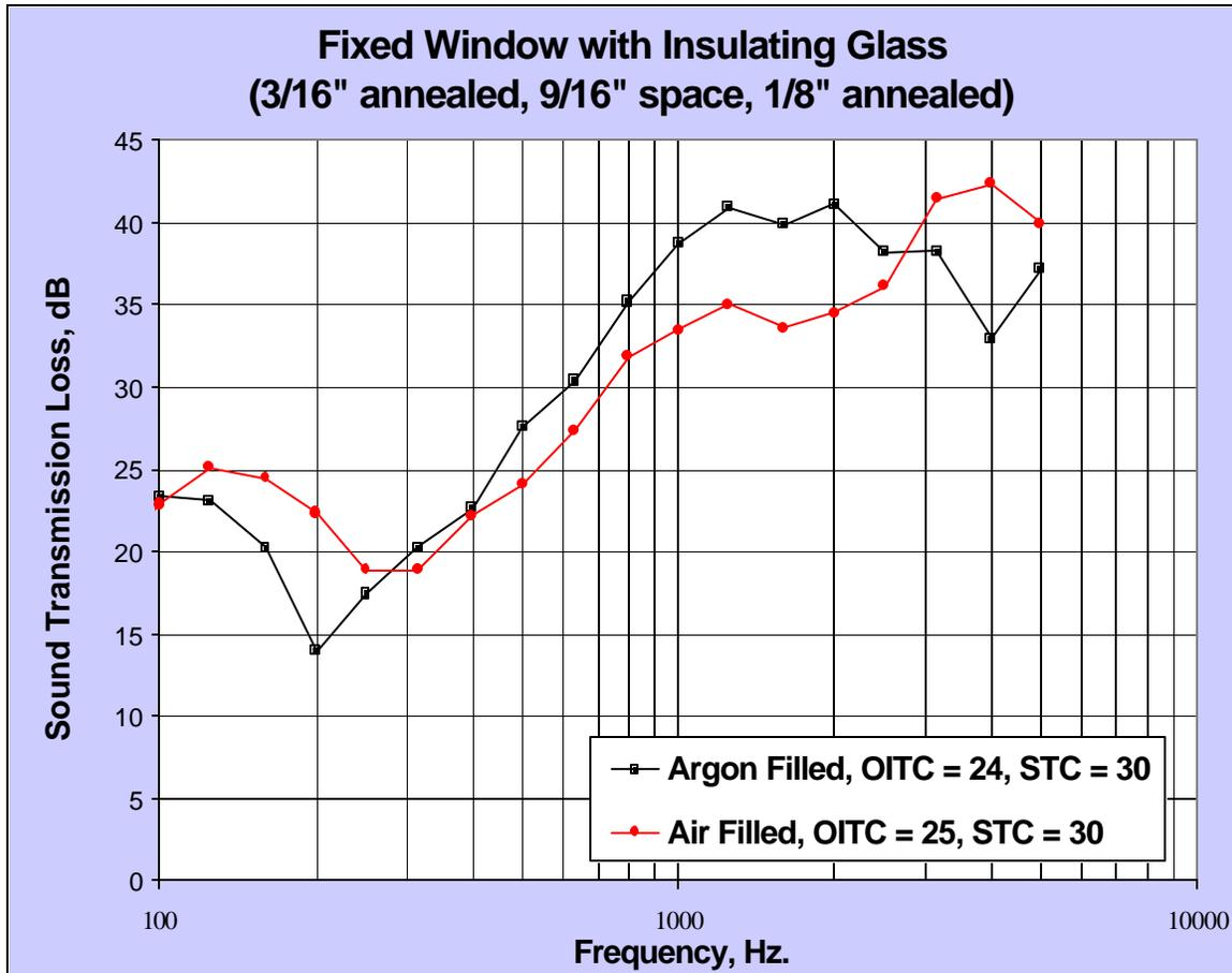
Figure 3.6 - Gas fill effect sound transmission loss
